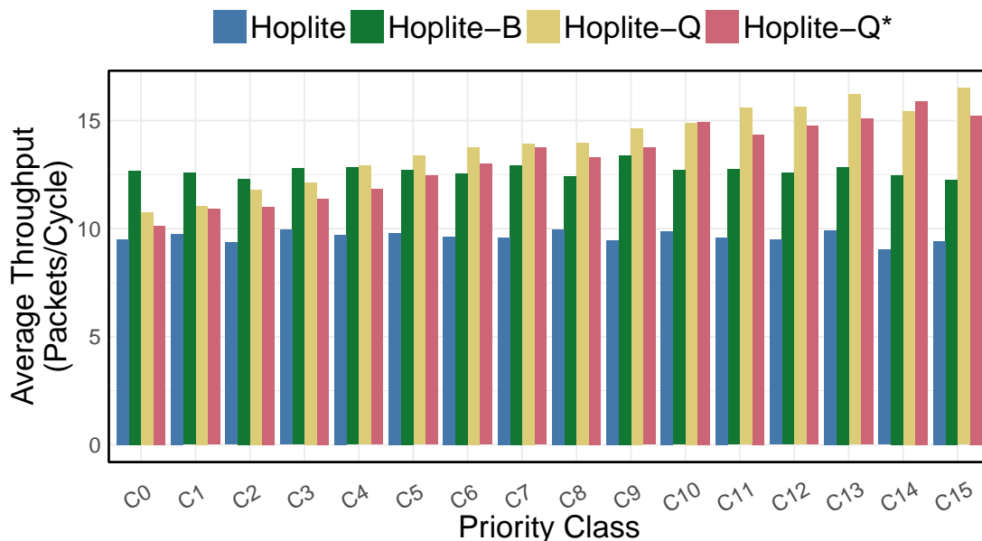
FIGURE 4.13: Average throughput of application in each priority class on 8 \times 8 NoC, where C = 16 and P = 16 .
